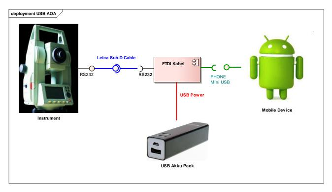
Currently, there's only one product available, the **Digitus DA-70160 USB2.0 - RS232 cable** utilising a FTDI FT312 chip. This cable needs an external power supply given by the battery pack.
